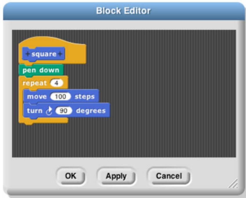
Your block appears at the bottom of the Motion palette. Here’s the block and the result of using it:
